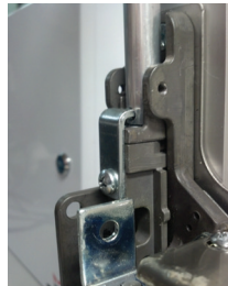
Rod fully extended and flush with bell crank. Retaining plate installed flat against bell crank with leg extending through rod and mating hole in bell crank.
